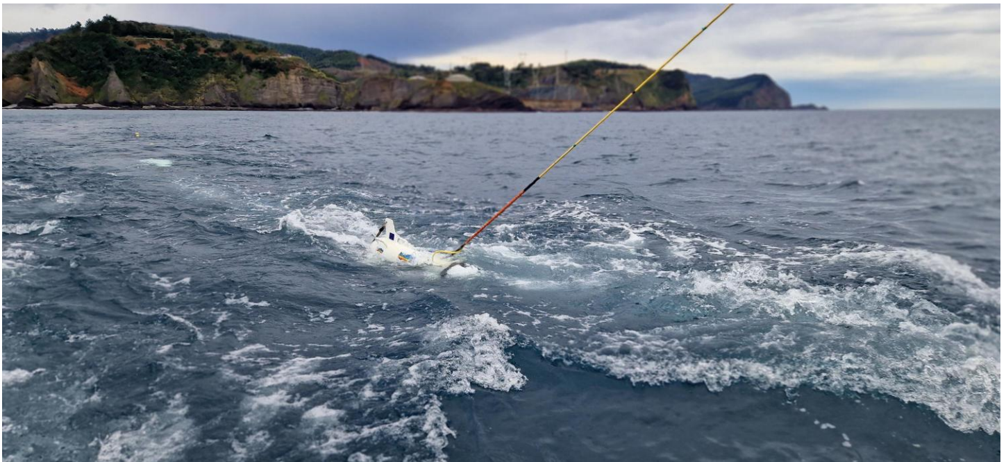
MAPPEM's vessel-towed 2D resistivity imaging system deployed near the coast. Image © Florent Colin.
